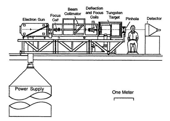
Figure 2.1. Experimental set-up for X-ray microbeam. Adapted from Abbs and Nadler (1987).
