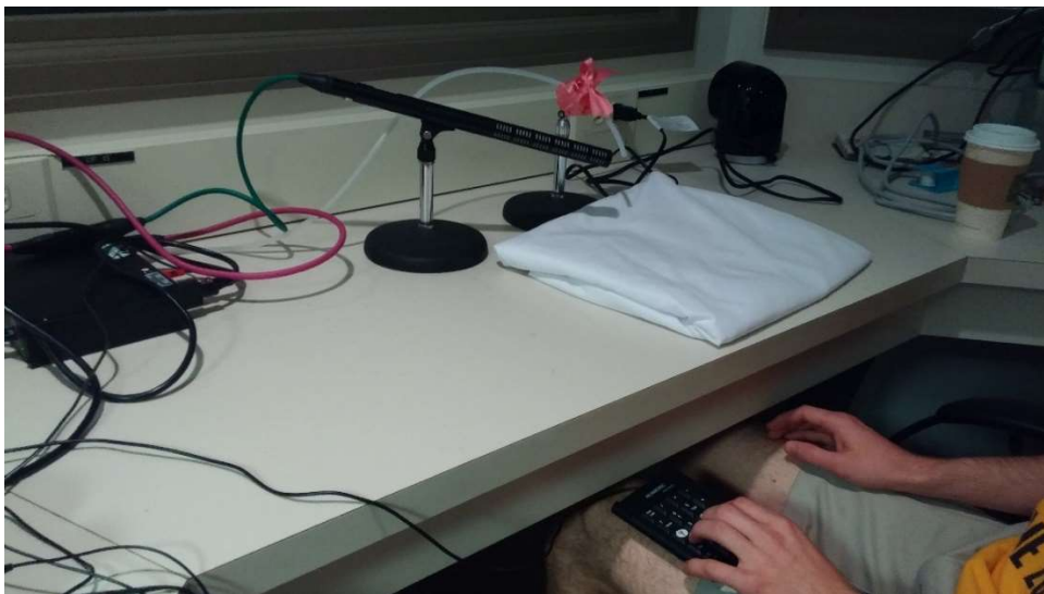
Figure 2.3b. Puff detection test setup: participant right hand positioned away from outflow of airtube. This test determines whether participant can detect airflow from cues other than tactile hand sensation.
