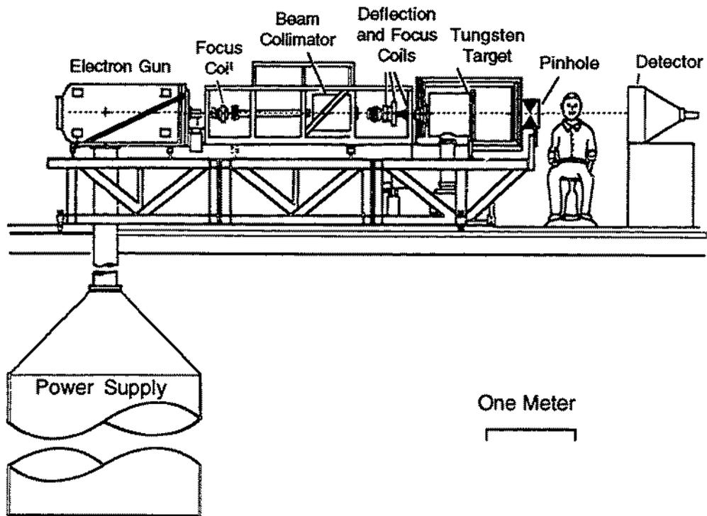
Figure 2.1. Experimental set-up for X-ray microbeam.
